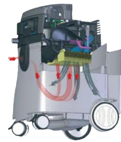
Air cycle during filter cleaning
