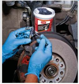
Lubricate all metal-to-metal contact points.
