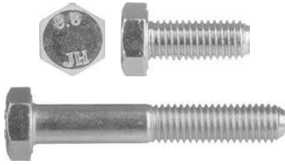
Bright Zinc Finish Class 8.8 Hex Head Cap Screws Din# 933 (Fully Threaded) Din# 931 (Partially Threaded)
